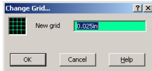
The **New Grid** field is where you specify the desired grid. You can specify independent X and Y axis grids by separating the two with a comma. Specifying only one value implies that both the X and Y grid will be the same.
