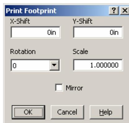
The **X-Shift** and **Y-Shift** fields are used to specify an offset for the footprint. The page origin is the lower-left of the page so positive X shifts are to the right and positive Y shifts are up.
