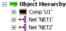
Only components and nets are listed directly under Object Hierarchy. Opening a component or net item will reveal component pins and net tracks respectively. RMB over an object and you will get a context menu that allows you to zoom to that object, delete that object, or edit/view its properties.
